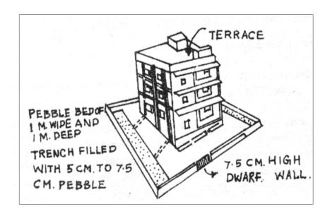
On the three sides along the inner periphery adjoining the compound wall, dig 1m. wide pit to a depth of 1.5 m. and fill it with 5 to 7.5 cm. sized pebbles let the rain water falling on the terrace flow into this pebble bed.
