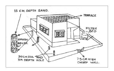
Dig a number of 3 m. deep and 30 cm dia percolation pits of 3 m. intervals around the plinth fill them up with broken bricks and pack the top 15 cm. with river sand Erect 7.5 c.m. high dwarf walls entrance to facilitate recharge.
